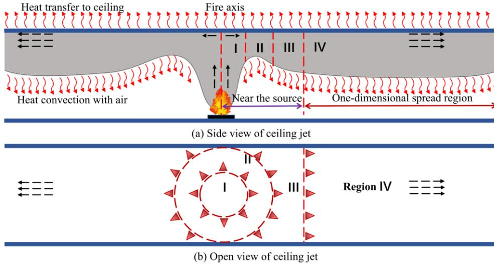
Fig. S5 Tunnel smoke flow diagram.
