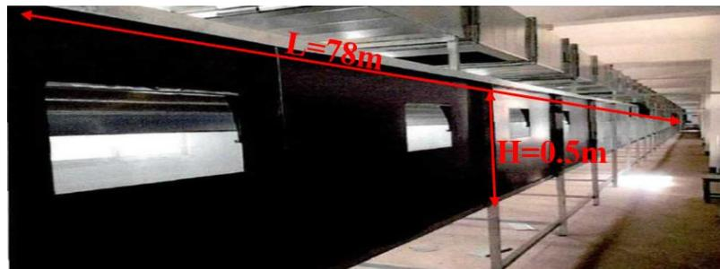
Fig. S3 Model tunnel experiment system.
