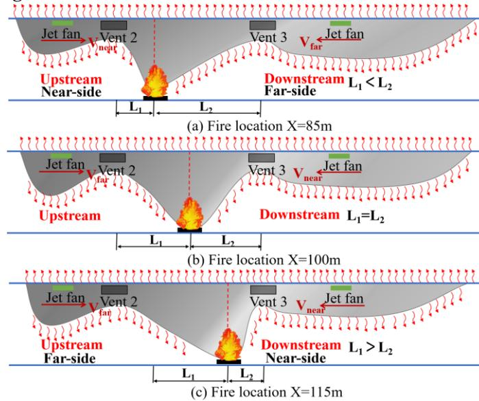
Fig. S1 Schematic diagram of the near-side and far-side of the smoke vent.
