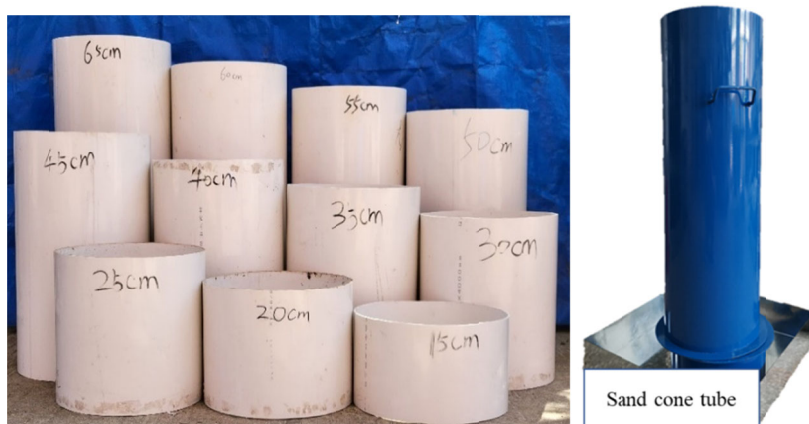
(a) PVC sand barrel (b) Steel sand barrel Fig. S1 Instruments to calibration the sand density
