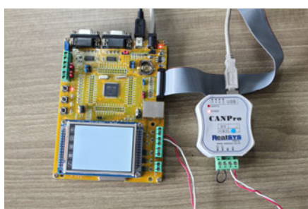
Fig. 9 Cortex M3 embedded test board
