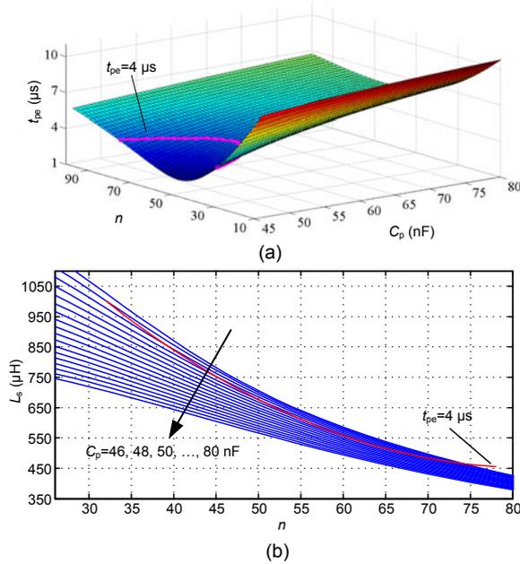
**Fig. 8** Design curves at variant  $C_p$  and  $n$ : (a)  $t_{pe}$ ; (b)  $L_s$ . References to color refer to the online version of this figure
