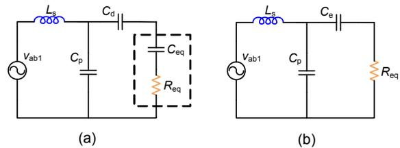
Fig. 4 Equivalent circuit of Fig. 2a in a steady condition (a) and the simplified circuit (b)
