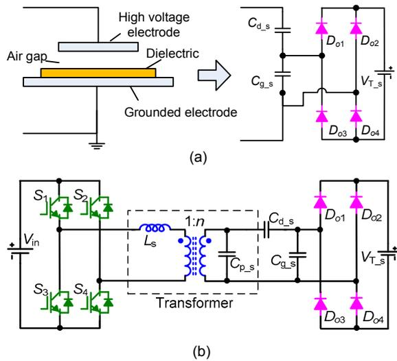
**Fig. 1** Equivalent circuits of DBD load (a) and the whole resonant converter (b)
