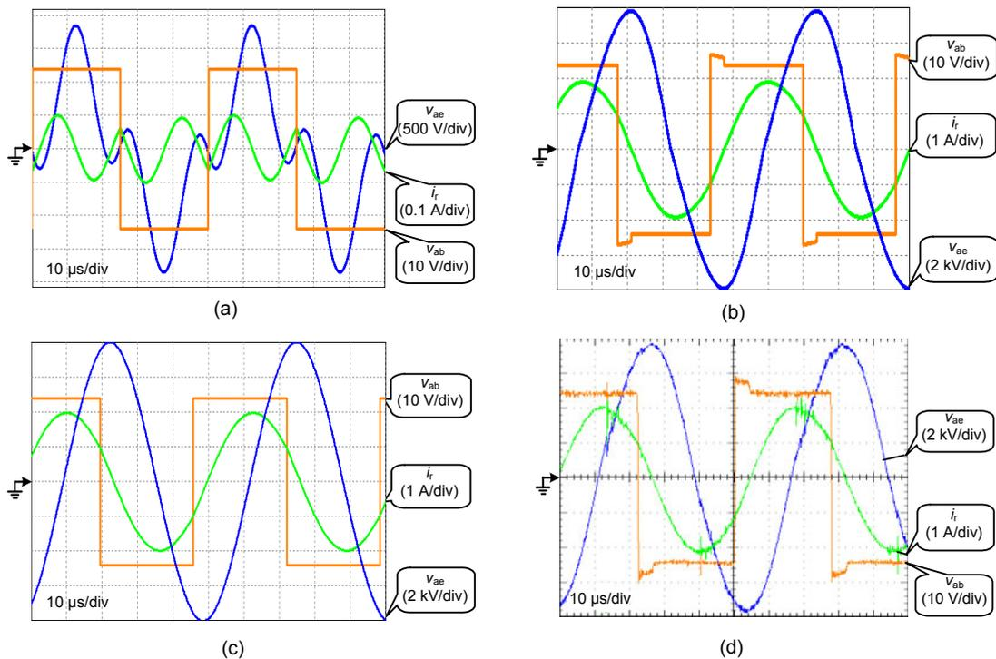
**Fig. 10 Waveforms of  $i_r$ ,  $v_{ab}$ , and  $v_{ae}$  in a rated condition in simulation without  $C_p$  (a), simulation from Fig. 1b (b), simulation with an equivalent model from Fig. 4b (c), and experiments (d)**
