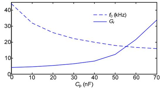
Fig. 5 Resonant frequency and tank gain with variant  $C_p$
