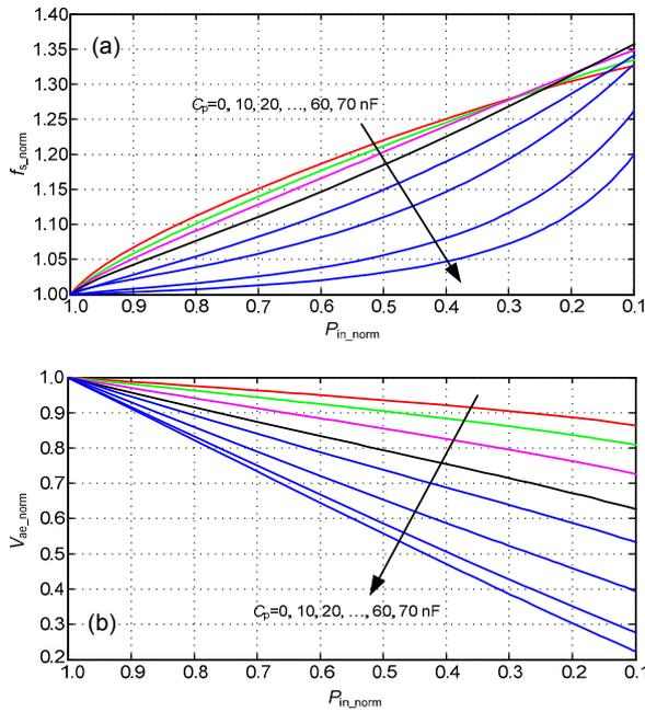
**Fig. 6 Performance comparison of variant  $C_p$  in the normalized frequency (a) and the normalized applied electrode voltage with PFM (b)**
