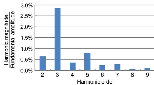
Fig. 12 Harmonic magnitude of experimental resonant current as a percentage of the fundamental amplitude in the rated condition
