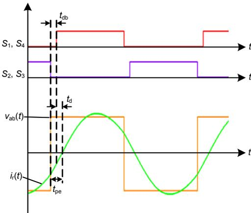
**Fig. 7 Zero-voltage switch (ZVS) waveforms**
