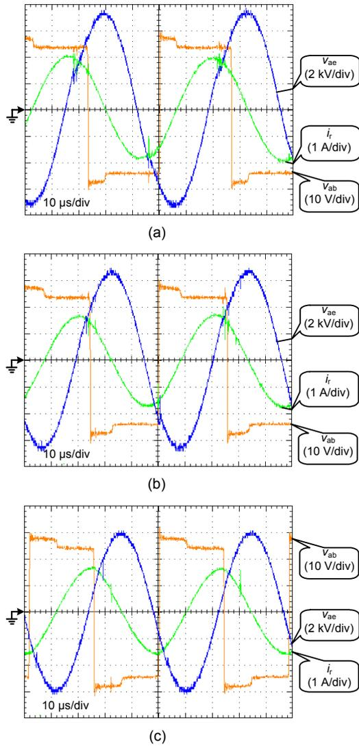
Fig. 11 Experimental waveforms when  $t_{pe}=6 \mu s$  (a),  $t_{pe}=8 \mu s$  (b), and  $t_{pe}=10 \mu s$  (c)
