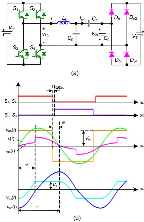
Fig. 2 Equivalent circuit of low power DBD referred to the primary side (a) and the key waveforms (b)
