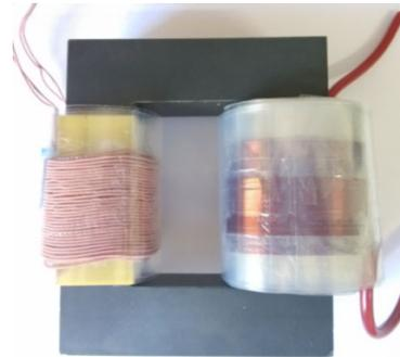
**Fig. 9** Transformer prototype
