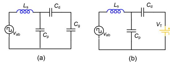
Fig. 3 Equivalent circuits when  $C_g$  is charging (a) and clamped (b)
