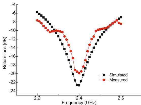
Fig. 13 Measured and simulated return loss characteristics
