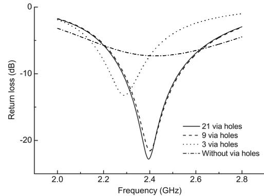
**Fig. 7** Return loss characteristic of the various number of via holes
