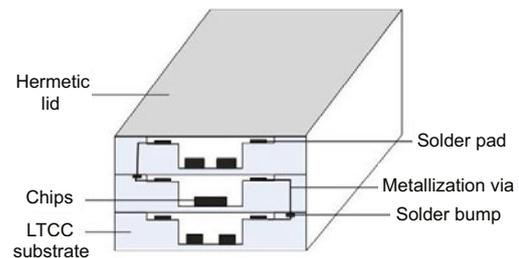
**Fig. 8** Illustration of the laminated LTCC MCM
