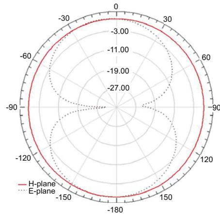
Fig. 4 Simulated E- and H-plane radiation patterns at 2.4 GHz
