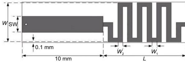
Fig. 1 Design parameters of the meander line antenna
