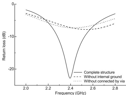
**Fig. 6** Return loss characteristic of different internal ground configurations
