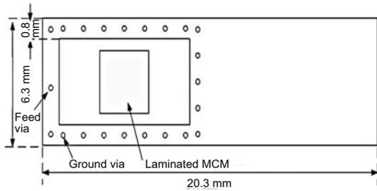
Fig. 9 Design parameters of the packaging layer
