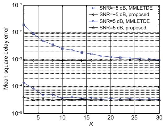
Fig. 8 Steady-state performance with  $2 \leq K \leq 30$  for narrowband signals ( $\mu = 1.0 \times 10^{-5}$ )
