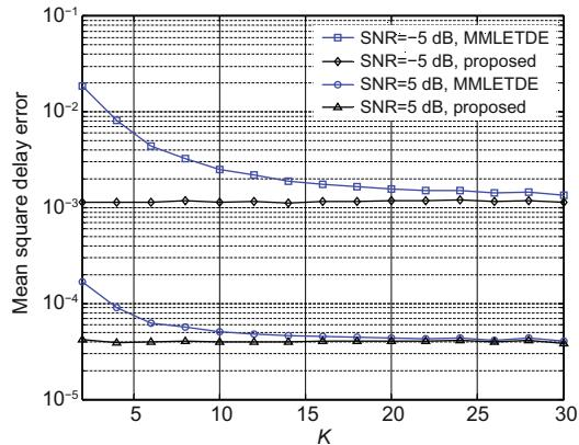
Fig. 7 Steady-state performance with  $2 \leq K \leq 30$  for sinusoidal signals ( $\mu = 1.0 \times 10^{-4}$ )
