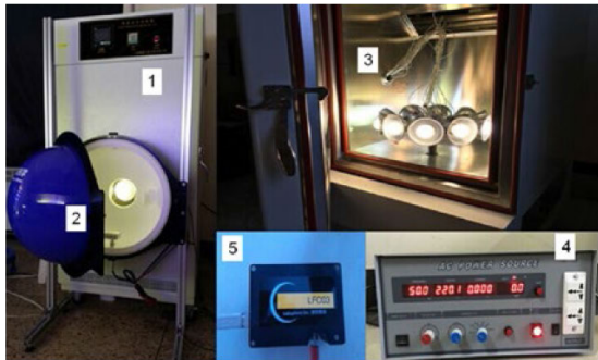
Fig. 1 Platform of the accelerated aging test for LED lamps
