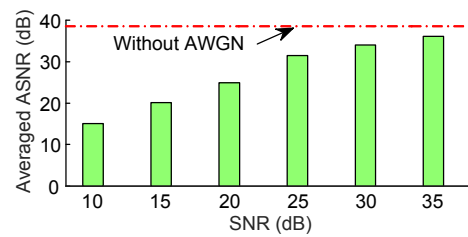
Fig. 8 Averaged auto-correlation sequence norm ratios (ASNRs) with and without AWGN
