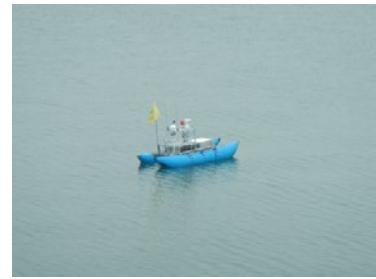
**Fig. 3 An unmanned surface bathymetry vehicle (USBV)**
