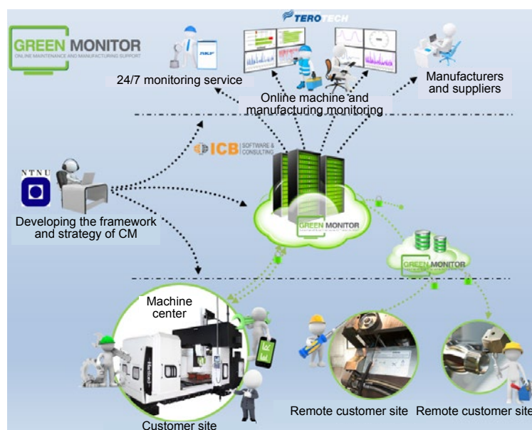
Fig. 4 Structure of the cognitive maintenance (CM) system in the Green Monitor Project
