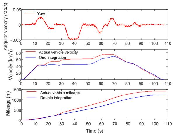
Fig. 16 Vehicle yaw angular velocity, speed, and location
