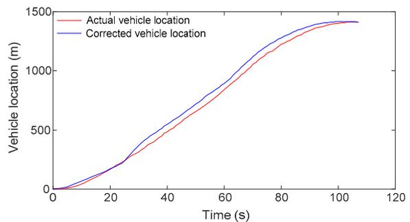
Fig. 17 Vehicle location after curve information correction
