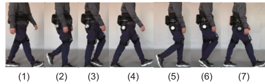
Fig. 10 Walking assistance with robotic exoskeleton
