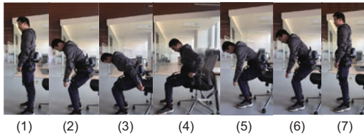
Fig. 17 A sit-to-stand cycle with exoskeleton assistance
