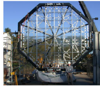
Fig. 9 The foldable diffractive primary lens with an aperture of 5 m
