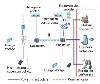
Fig. 1 A simplified framework of smart grid
