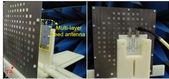
**Fig. 11** Fabricated prototype of the monopulse transmitarray antenna (TA: transmitarray)
