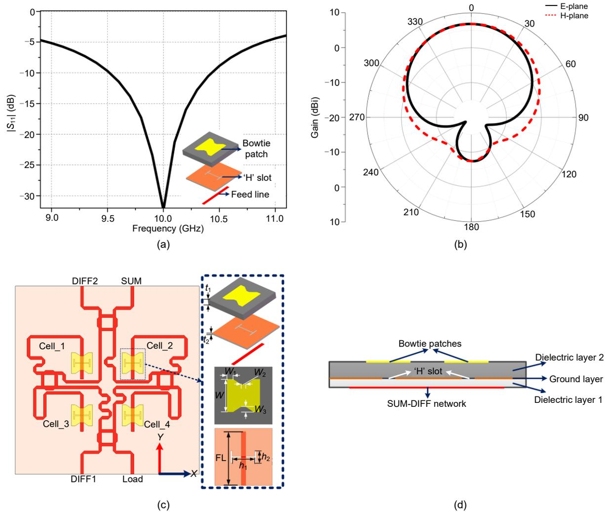
Fig. 2  $|S_{11}|$  (a) and radiation patterns (b) of the aperture-coupled microstrip antenna unit cell and top view (c) and side view (d) topology of the multi-layer feed antenna based on the aperture-coupled microstrip antenna ( $W_1=1.5$  mm,  $W_2=1$  mm,  $W_3=1.3$  mm,  $W=8$  mm,  $h_1=5.5$  mm,  $h_2=3$  mm,  $FL=13.2$  mm,  $t_1=2$  mm,  $t_2=0.5$  mm)
