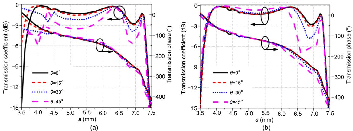
**Fig. 7 Transmission coefficient and transmission phase of transmitarray unit cells under oblique incidences with TE polarization (a) and TM polarization (b)**
