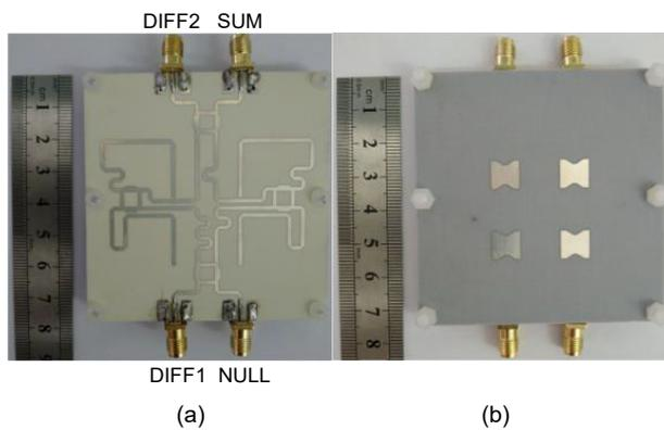
Fig. 3 Fabricated prototype of the multi-layer feed antenna: (a) SUM-DIFF network layer; (b) aperture-coupled microstrip antenna layer
