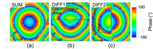
Fig. 15 E-field phase distributions of the feed antenna at a distance of 100 mm when the SUM (a), DIFF1 (b), and DIFF2 (c) ports are excited (the size of the observation plane is  $240\text{ mm}\times 240\text{ mm}$ )
