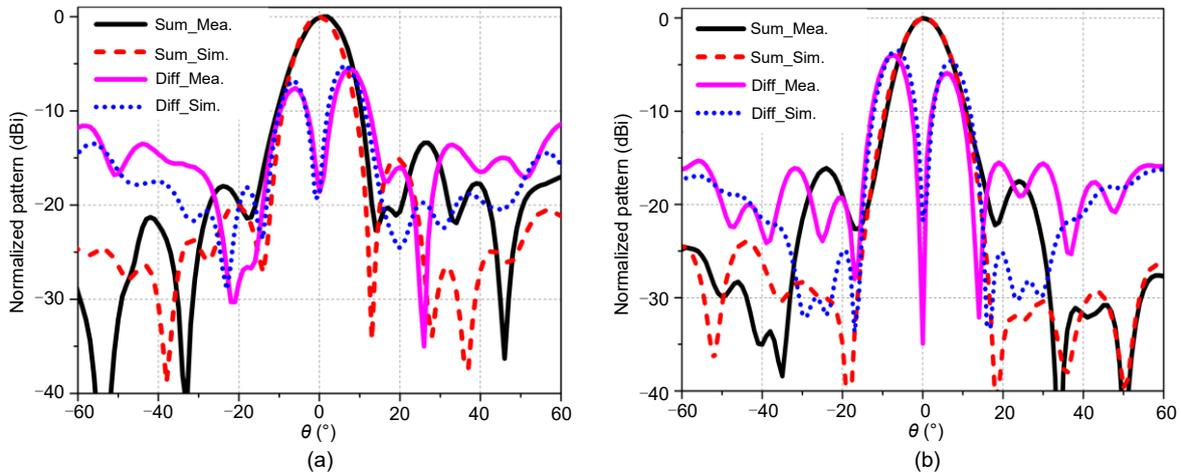
Fig. 13 Normalized far-field sum-difference (Sum-Diff) patterns in simulation (Sim.) and measurement (Mea.) in the E-plane (a) and H-plane (b)
