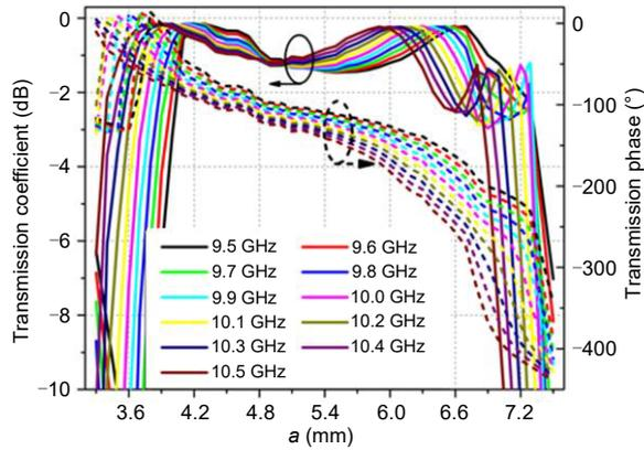
**Fig. 8** Transmission coefficient and transmission phase of transmitarray unit cells of different sizes as a function of frequency
