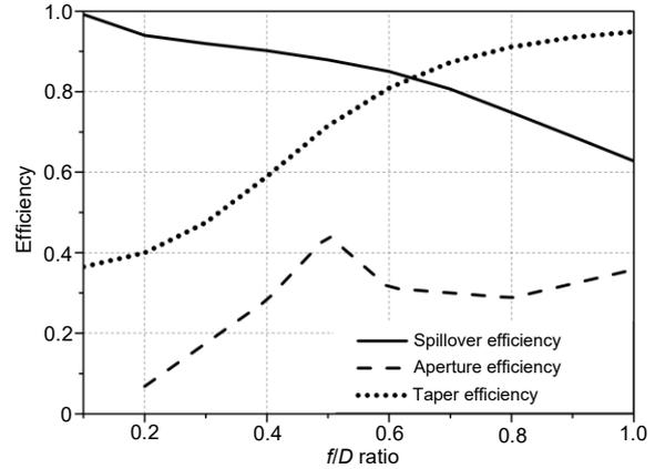
**Fig. 10** Spillover, taper, and aperture efficiencies versus the  $f/D$  ratio
