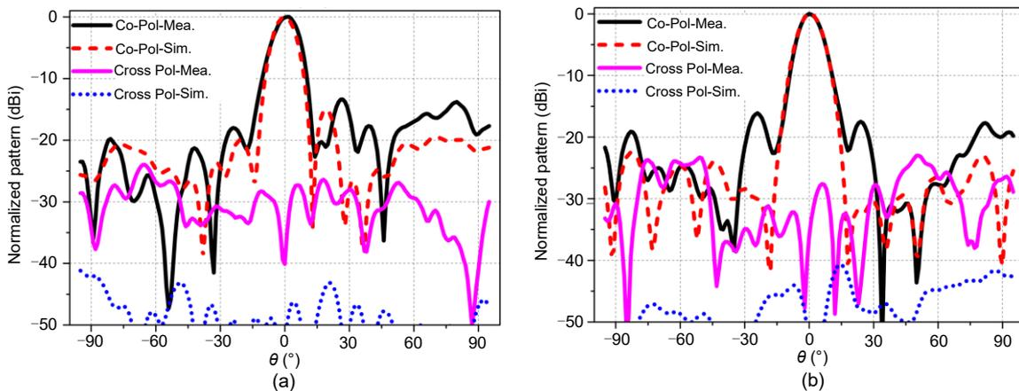
**Fig. 12** Co-polarized (Pol) and cross-polarized sum pattern comparison between simulation (Sim.) and measurement (Mea.) in the E-plane (a) and H-plane (b)
