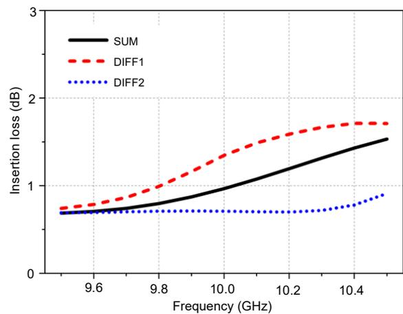
Fig. 4 Simulated insertion losses from the SUM, DIFF1, and DIFF2 ports to the four ports of the antenna elements
