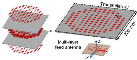
**Fig. 9** Topology of the monopulse transmitarray antenna
