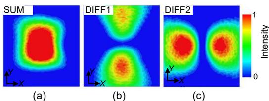
Fig. 14 E-field intensity distributions of the feed antenna at a distance of 100 mm when the SUM (a), DIFF1 (b), and DIFF2 (c) ports are excited (the size of the observation plane is  $240\text{ mm}\times 240\text{ mm}$ )
