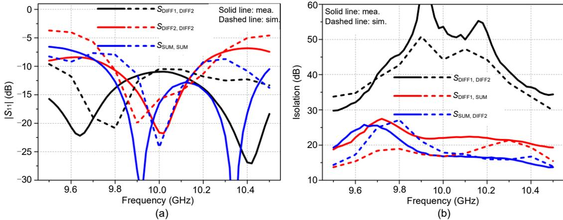
Fig. 5 Simulated (sim.) and measured (mea.)  $|S_{11}|$  of sum port SUM, difference ports DIFF1 and DIFF2 of the multi-layer feed antenna (a) and simulated and measured isolation between the SUM, DIFF1, and DIFF2 ports (b) References to color refer to the online version of this figure
