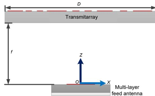
**Fig. 1 Configuration of the X-band monopulse transmitarray antenna**
