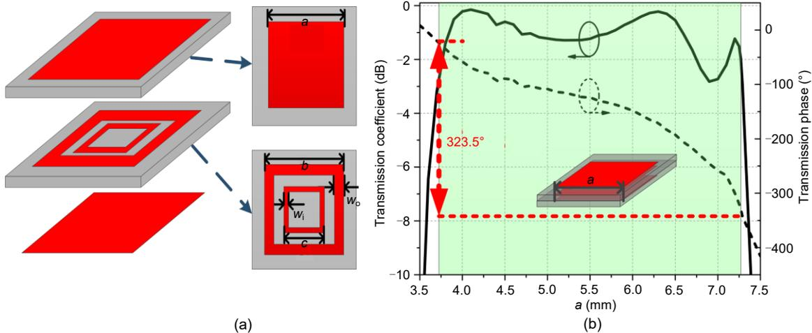
Fig. 6 Layout of the two-layered transmitted unit cell (a) and transmission coefficient and transmission phase of the transmitted element (b)
