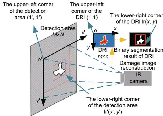
Fig. 7 Schematic of damage characteristic area localization
