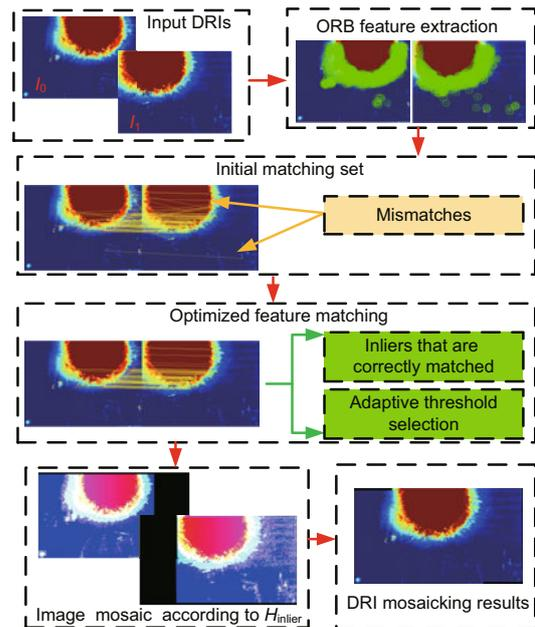
**Fig. 4** Schematic of the image mosaicking scheme
