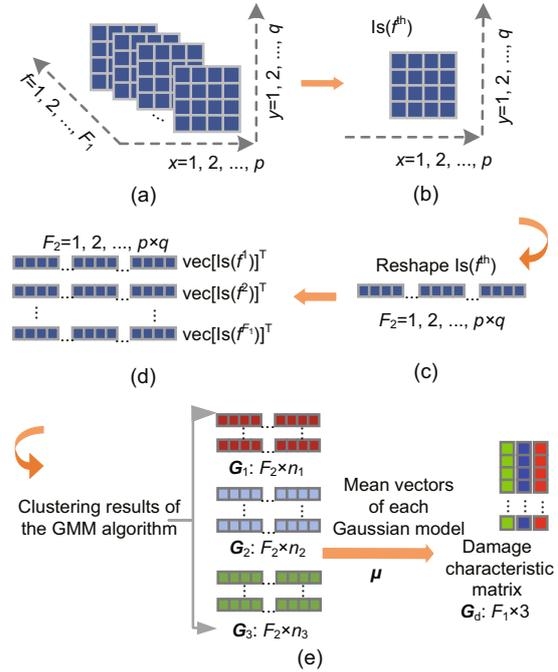
Fig. 2 Schematic of the data conversion and clustering: (a) image sequence  $Is(f)$ ; (b)  $f^{th}$  frame of  $Is(f)$ ; (c)  $vec[Is(f^{th})]^T$ ; (d) reconstruction matrix  $O_{ttr}$ ; (e) damage characteristic matrix construction
