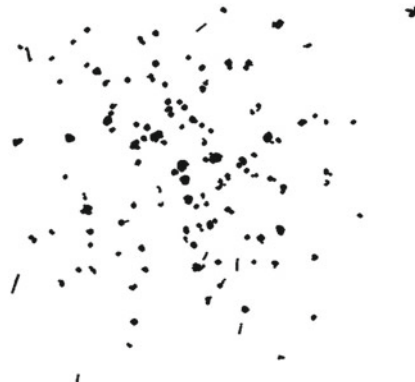
Fig. 14 All craters in the image of the rear wall (the size is 2000 mm × 2000 mm)
