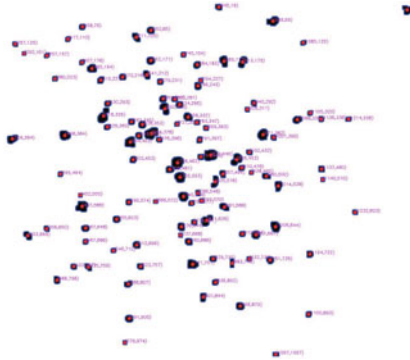
Fig. 16 Centroids of contours of craters in Fig. 15 (the size is 2000 mm × 2000 mm)
