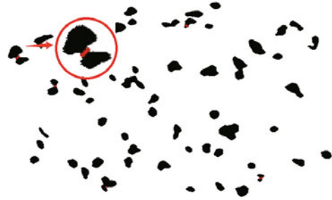
Fig. 8 Results of Fig. 7a by concave point segmentation (the size is 80 mm × 53 mm). References to color refer to the online version of this figure
