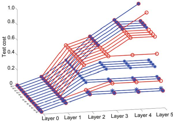
Fig. 4 Test cost on real-world applications (The red lines refer to the test cost of AO\*-based methods and the blue lines refer to the test cost of HP-based methods. References to color refer to the online version of this figure)
