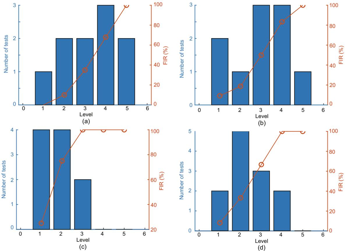
**Fig. 1** Fault isolation rate (FIR) improvement and test assignment on the anti-tank system dataset: (a) sequential strategy; (b) MAO\*-based strategy; (c) HP-based strategy; (d) Rollout-HP-based strategy
