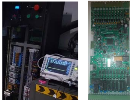
Fig. 7 Elevator control system for gearless and hydraulic configurations, developed using XIRAC OS for precision task scheduling and safety-critical operations
