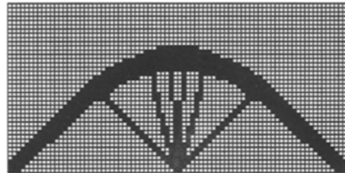
Fig.5 Optimum configuration for the Michell type structure
