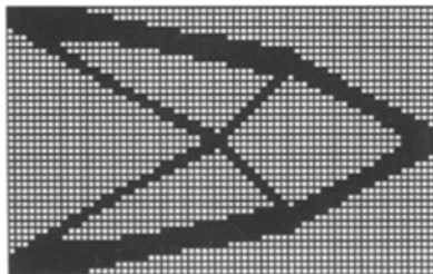
Fig.3 Optimum configuration for the short cantilever
