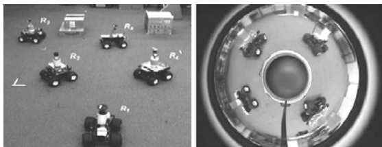
Fig.4 A formation of five car-like robots (left) and a sample image from omni-directional camera (right)
