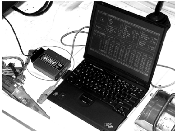
Fig.4 Adjustment of engine input parameters using MoTeC M4 programmable ECU
