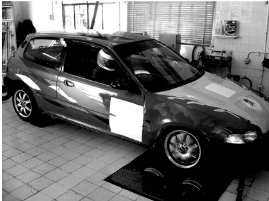
Fig.5 Car engine performance data acquisition on a chassis dynamometer
