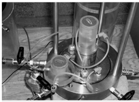
Fig.3 Triaxial cell equipped with bender element
