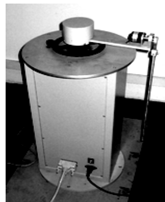
Fig.3 Rotary inverted pendulum apparatus
