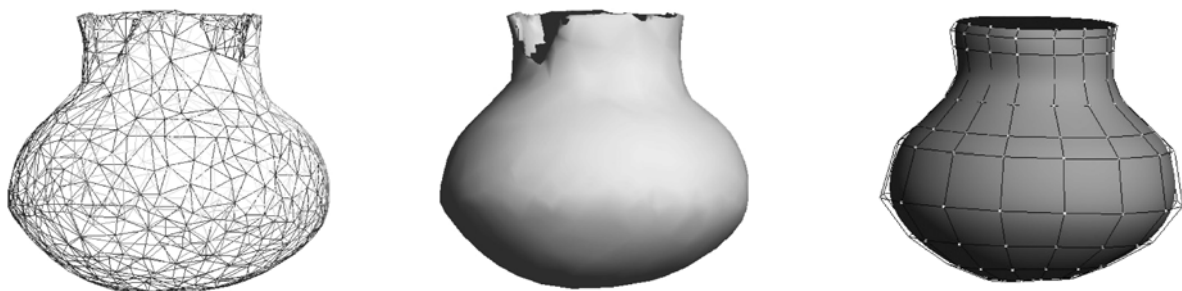
Fig.4 (L to R) A scanned vessel rendering by wire frame and shading, and its surface model generated by least squares approximation
