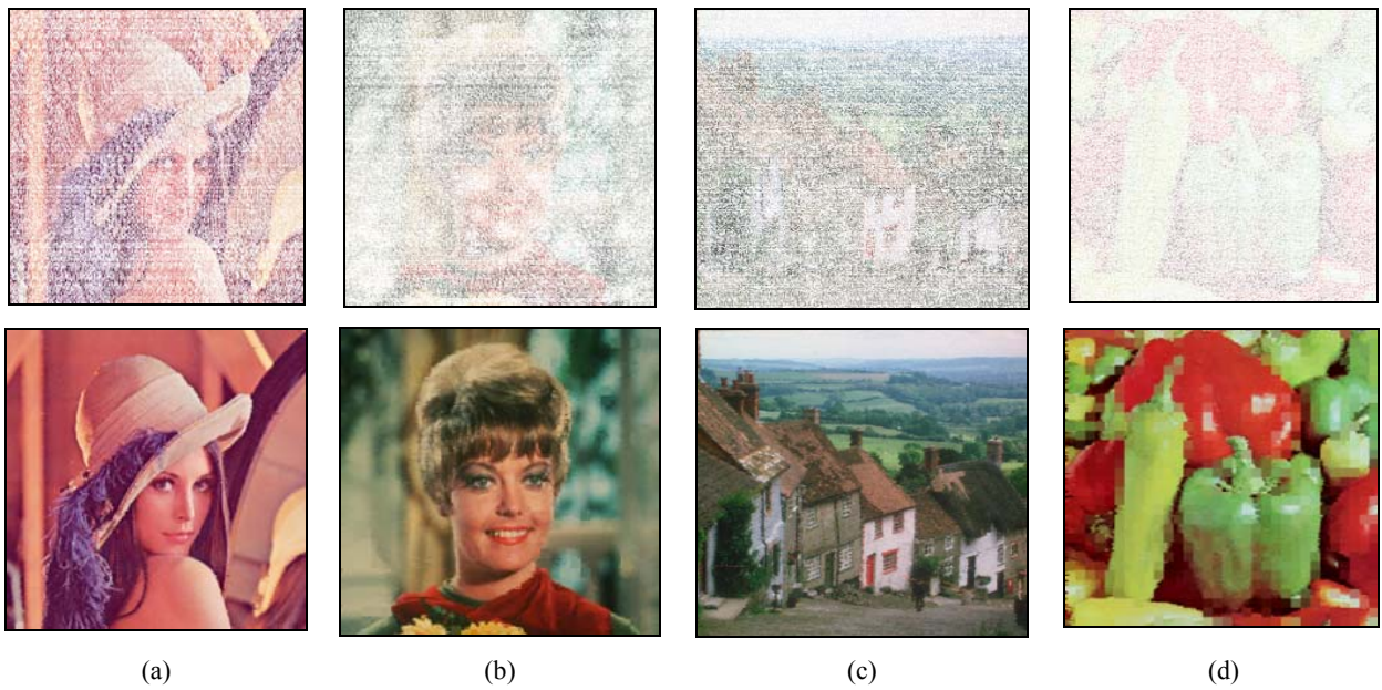
Fig.4 Experimental results in different noise conditions (a) Noise ratio=61.2%, PSNR =30.1 dB; (b) Noise ratio=73.1%, PSNR =28.16 dB; (c) Noise Ratio=80.6%, PSNR =30.9 dB; (d) Noise Ratio=90.3%, PSNR =22.1 dB
