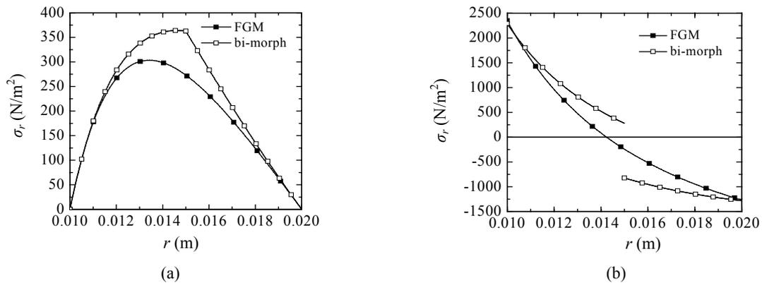
**Fig.2** The normal stress  $\sigma_r$  (a) and  $\sigma_\theta$  (b) of the cylinder in different analytical models at  $V=100$  V
