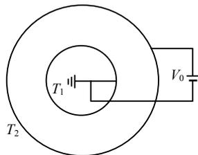
Fig.1 The graded hollow cylinder subjected to thermal and electric loading
