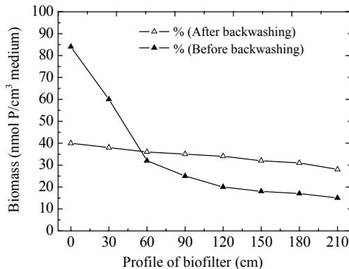
Fig.3 Biomass along the profile of biofilter
