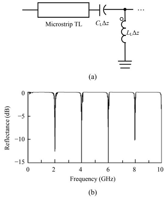
**Fig.4** (a) Circuit diagram of the alternate-layered structure; (b) The reflectance as a function of frequency for a DBR consisting of ideal microstrip RHTL and lumped element LHTL layers (40 layers in all), with  $EL_R=\pi$ ,  $\eta_R=1 \Omega$  and  $EL_L=-\pi$ ,  $\eta_L=2 \Omega$
