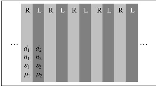
Fig.1 Structure of an RHM-LHM multilayered Bragg reflector
