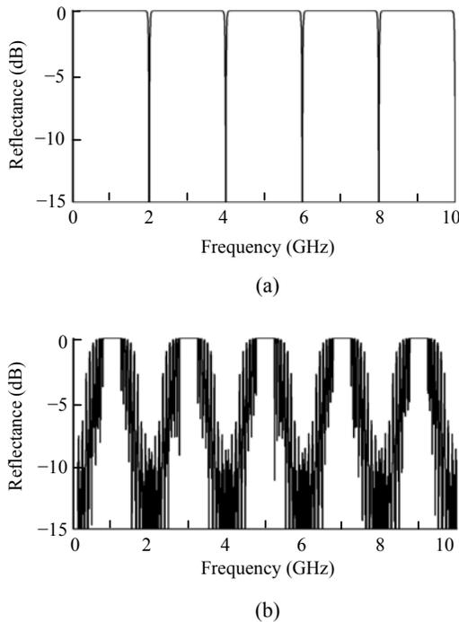
**Fig.3** The reflectance as a function of frequency for a DBR consisting of ideal microstrip RHTL and LHTL layers (totally 40 layers). (a) For the case of RHTL-LHTL period with  $EL_R=\pi$ ,  $\eta_R=1 \Omega$  and  $EL_L=-\pi$ ,  $\eta_L=2 \Omega$ ; (b) For the case of dual RHTL period with  $EL_{R1}=\pi$ ,  $\eta_{R1}=1 \Omega$  and  $EL_{R2}=\pi$ ,  $\eta_{R2}=1 \Omega$
