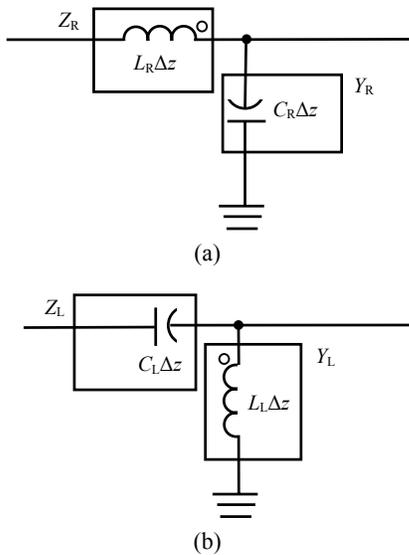
Fig.2 Transmission line units: (a) Right-handed transmission line (RHTL) unit and (b) Left-handed transmission line (LHTL) unit
