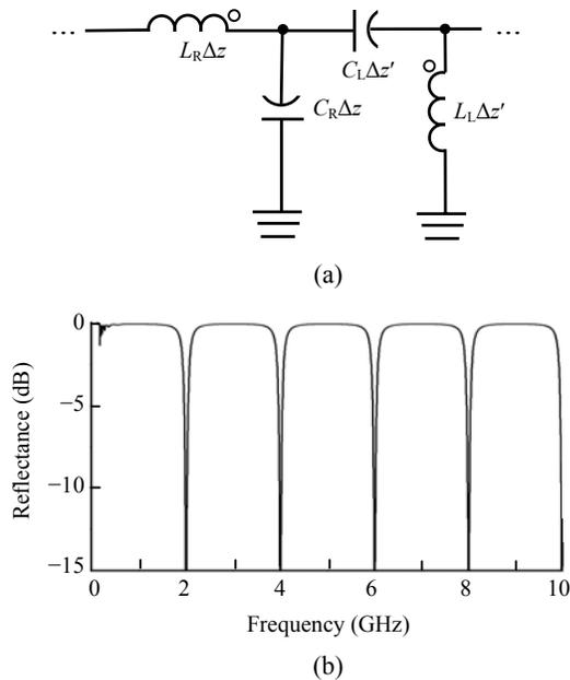
**Fig.5** (a) The circuit diagram of the alternate-layered structure; (b) The reflectance as a function of frequency for a DBR consisting of L-C lumped-element RHTL (period with  $EL_R = \pi$ ,  $\eta_R = 20 \Omega$ , 1 layer of 50 units) and LHTL layers (period with  $EL_L = -2\pi$ ,  $\eta_L = 1 \Omega$ , 1 layer of 10 units)
