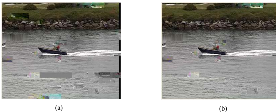
Fig.6 First frame of Coastguard sequence with CAVLC. (a) UDP-Lite2+RoHC at BER 1e-3; (b) UDP-Lite2+RoHC+FEC at BER 1e-3
