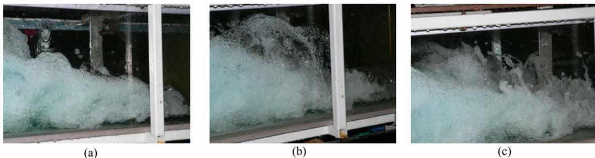
**Fig.5 High-shutter photographs of instantaneous spray/splash structures.  $Fr_1=8.6$ ,  $d_1=0.024$  m,  $V_1=4.1$  m/s,  $x_1=1$  m, flow from right to left (shutter 1/1000 s). (a) Side view of the roller; (b) Details of some instantaneous air-water projections; (c) Details of the instantaneous roller free-surface**
