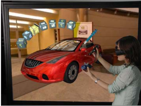
Fig.1 Material manipulation of a VR model, provided by MEMPHIS, in a VR system (in-house solution TiciView, image source: Hur et al. , 2006)
