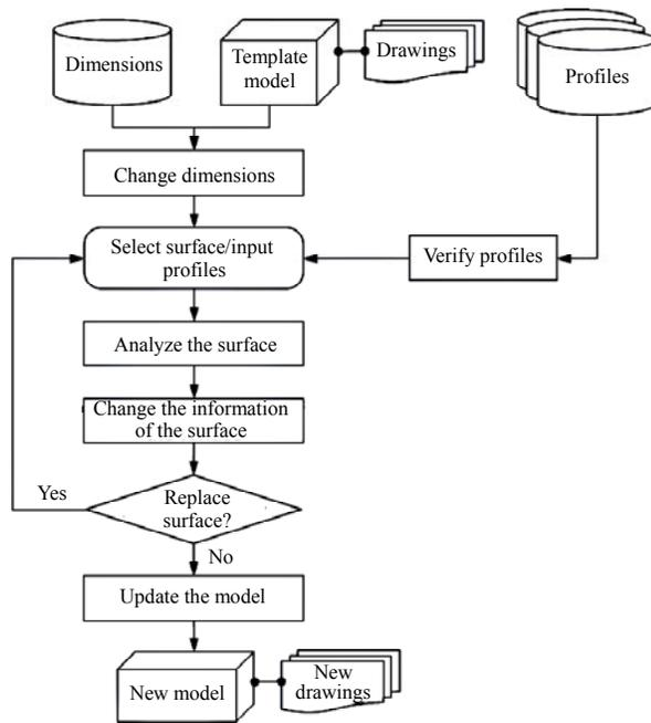
Fig.6 The procedure of parametric design of PFFSs
