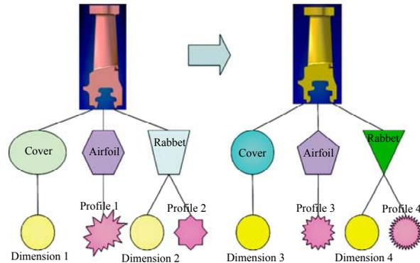
Fig.2 Generation of new model by replacing dimensions and profiles
