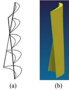
Fig.10 A 3D airfoil model. (a) Profiles; (b) Solid model
