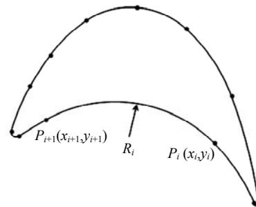
Fig.9 A profile for an airfoil
