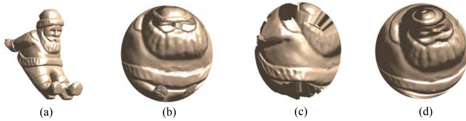
Fig.1 The parametrization process of Santa Claus. (a) The model; (b) The initial map; (c) The result after one step computing; (d) The final spherical parametrization
