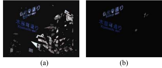
Fig.6 Effect of SVM. (a) Input: CCs accepted by cascade; (b) Output: CCs accepted by SVM
