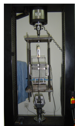
Fig.3 Setup of pullout test. (a) Sketch; (b) Photo
