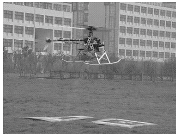
Fig.2 Fully equipped mini unmanned helicopter in flight for landmark detection
