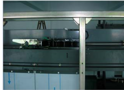
Fig.7 Prototype of the motor and the elevator door
