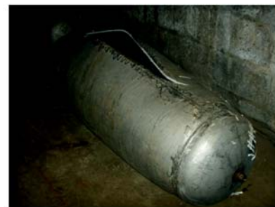
Fig.10 Specimen after burst
