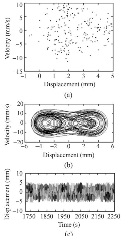
**Fig.4** Poincare map (a), phase diagram (b) and wave diagram (c) of displacement ( $p=252$  N/m<sup>2</sup>)
