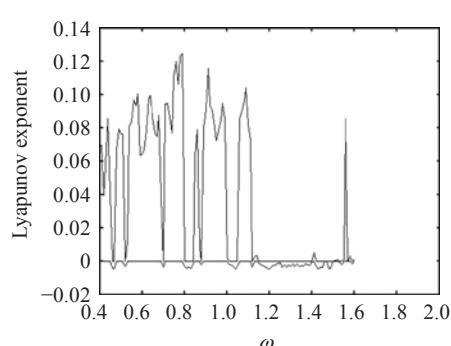
**Fig.18** Lyapunov exponent diagram ( $p=100 \text{ N/m}^2$ ,  $B_z=1.0 \text{ T}$ )
