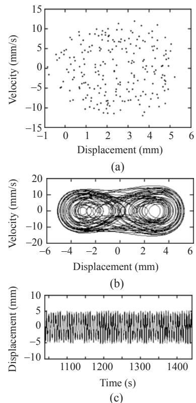
**Fig.9** Poincare map (a), phase diagram (b) and wave diagram (c) of displacement ( $B_z=0.5 \text{ T}$ )
