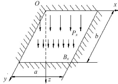
**Fig.1 Model of thin rectangular plate**
