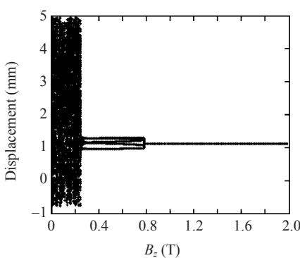
**Fig.19 Bifurcation diagram ( $\omega_0=1.0$ ,  $p=100$  N/m $^2$ )**
