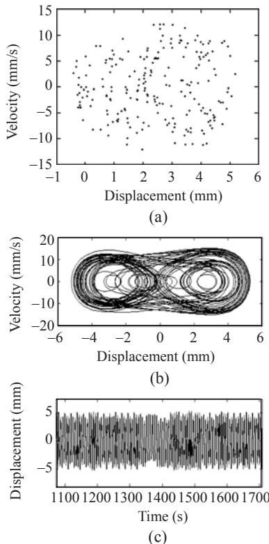
**Fig.6** Poincare map (a), phase diagram (b) and wave diagram (c) of displacement ( $p=266 \text{ N/m}^2$ )
