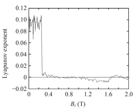
**Fig.20** Lyapunov exponent diagram ( $\omega_0=1.0$ ,  $p=100 \text{ N/m}^2$ )
