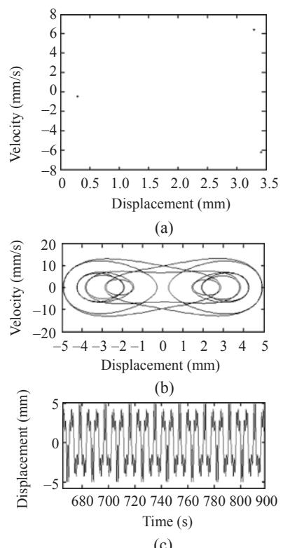
**Fig.5** Poincare map (a), phase diagram (b) and wave diagram (c) of displacement ( $p=256$  N/m<sup>2</sup>)
