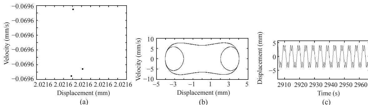
Fig.14 Poincare map (a), phase diagram (b) and wave diagram (c) of displacement ( $\omega_0=1.3$ )
