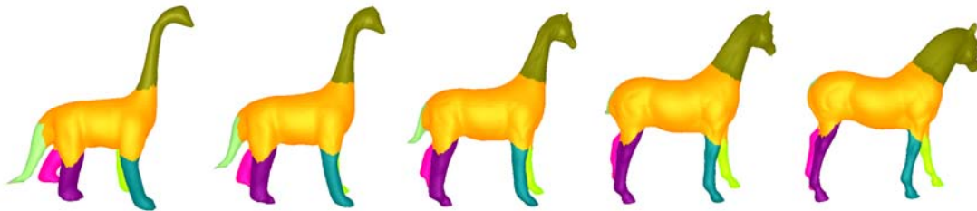
Fig.8 Mesh interpolation between a dinosaur and a horse
