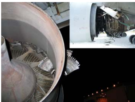
Fig.1 A CF6 Aeroengine turbine disk burst accident
