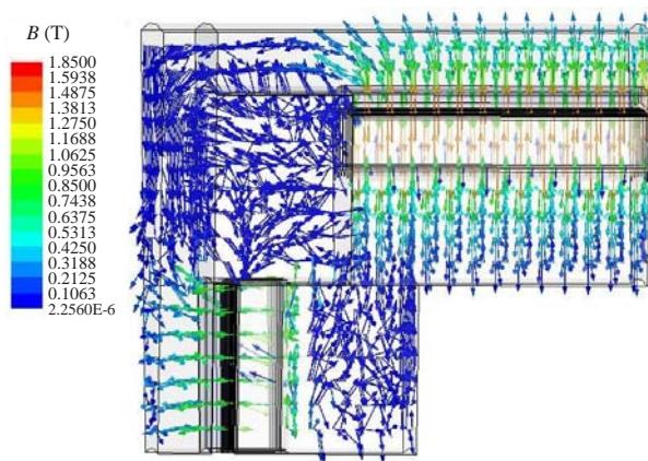
Fig.4 Plot of magnetic flux density vector
