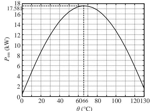
**Fig.2 Power-angle curve of the model machine**
