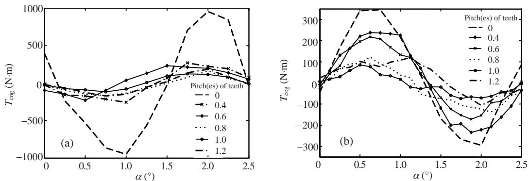
**Fig.6** Comparison of cogging torque ( $T_{\text{cog}}$ ) and angle of skewed PM in a cylindrical electric machine (a) and a disk electric machine (b)
