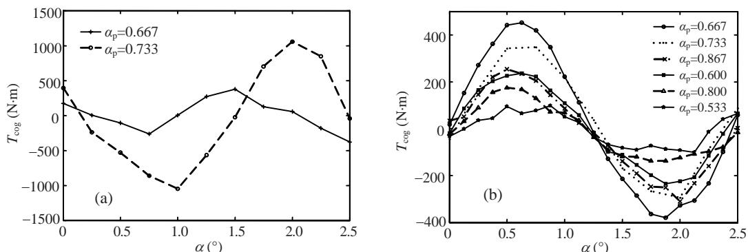
**Fig.5** Comparison of cogging torque ( $T_{\text{cog}}$ ) and  $\alpha_p$  in a cylindrical electric machine (a) and a disk electric machine (b)
