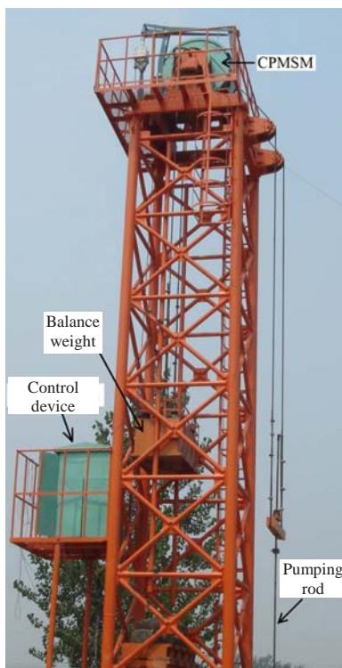
**Fig.7** Photograph of the direct-drive pumping unit installed in an existing oil well
