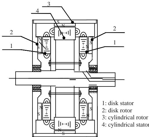
Fig.1 Structure of the compound permanent magnet synchronous machine (CPMSM)
