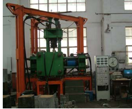
Fig. 1 Dynamic-static triaxial electronic hydraulic servo test system
