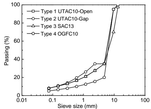
**Fig. 2** Aggregate gradations for four types of AC
