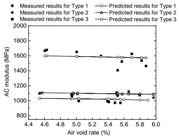
**Fig. 3 Measured and predicted results of AC modulus for Types 1–3**
