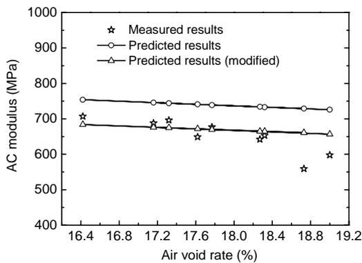
Fig. 5 Measured and predicted results for Type 4
