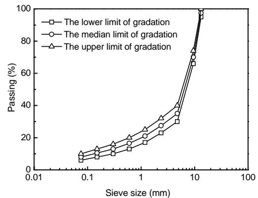
Fig. 9 Aggregate gradation for Type 3
