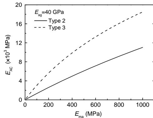
Fig. 7 Effect of elastic modulus of matrix on elastic modulus of AC
