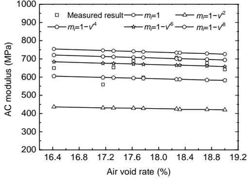
Fig. 4 Effect of debonding on the modulus of Type 4
