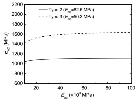
Fig. 6 Effect of elastic modulus of aggregate on elastic modulus of AC
