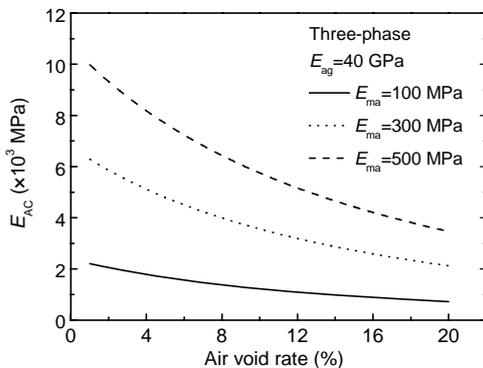
Fig. 8 Effect on elastic modulus of AC by air void
