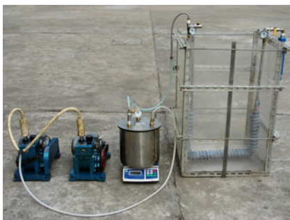
Fig. 10 Photo of the sludge dewatering with aeration-vacuum model test device
