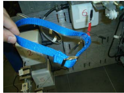
Fig. 8 An end-effector interface for CATRASYS on an ankle application at LARM in Cassino (Grande, 2008)
