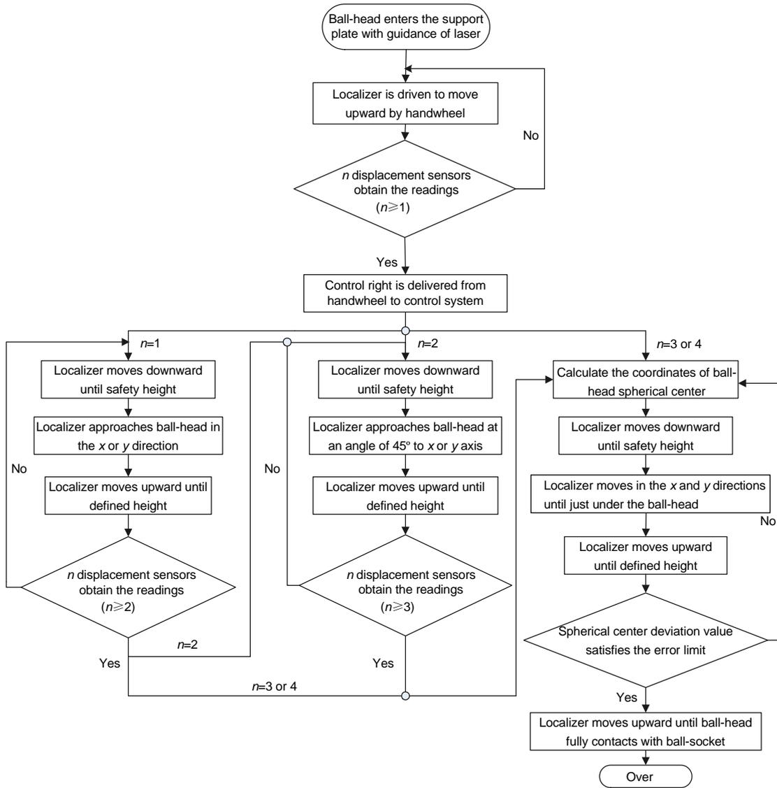
Fig. 6 Algorithm flowchart
