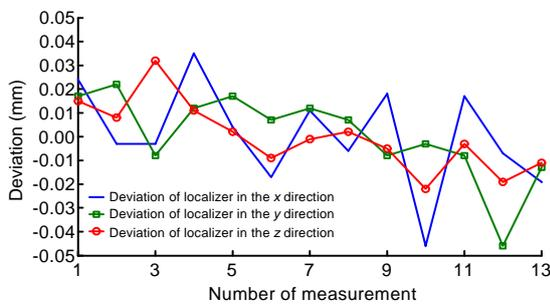
**Fig. 10** Positional deviation of the localizer while contacted completely
