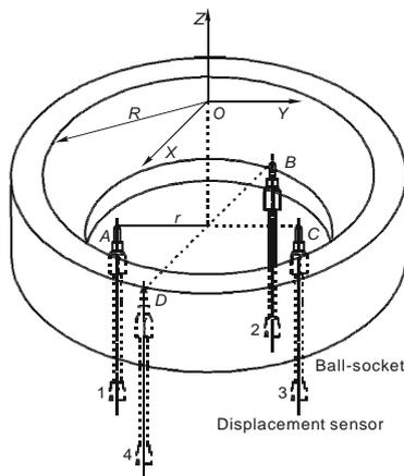
Fig. 4 Arrangement of displacement sensors
