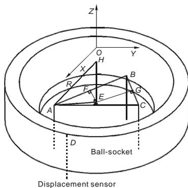
Fig. 7 Spherical center calculation of the ball-head
