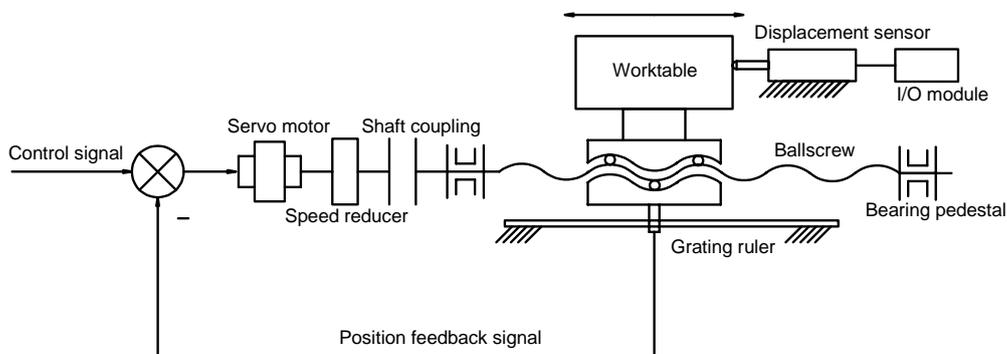
**Fig. 3** Calibration of displacement sensors
