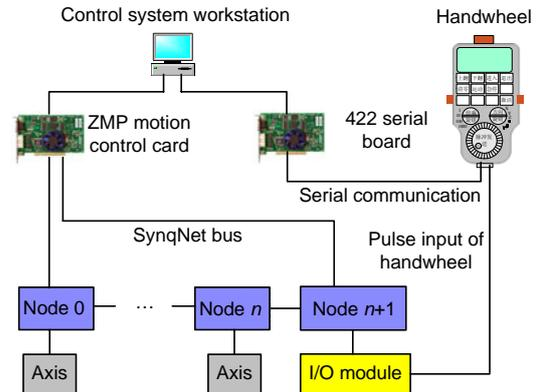
Fig. 2 Relation between the handwheel and the control system
