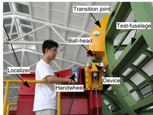
Fig. 8 Device for large aircraft components gaining accurate support by ball joint
