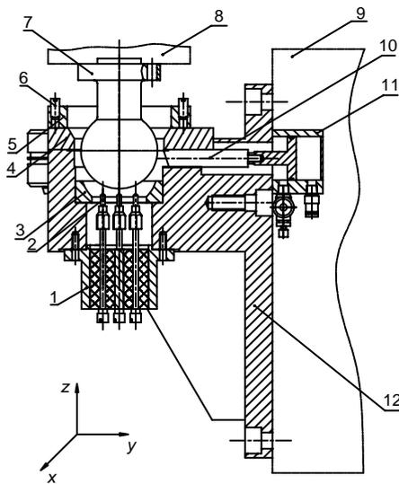
1: Sensor fixation apparatus; 2: Displacement sensor; 3: Ball-socket; 4: Pressure plate; 5: Laser emitter support; 6: Laser emitter; 7: Ball-head; 8: Transition joint; 9: Localizer; 10: Locking pin; 11: Fine lock cylinder; 12: Support plate
