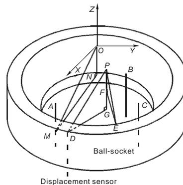
Fig. 5 Mounting height calculation model of displacement sensors
