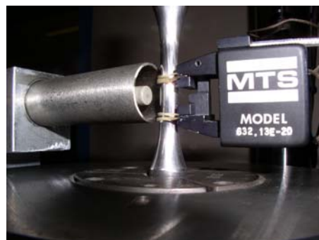
Fig. 1 Experimental setup of extensometer and fluxgate magnetometer. The magnetometer probe was shielded by a cylindrical Mu metal tube to reduce the magnetic interference. Rubber bands were used to install the extensometer
