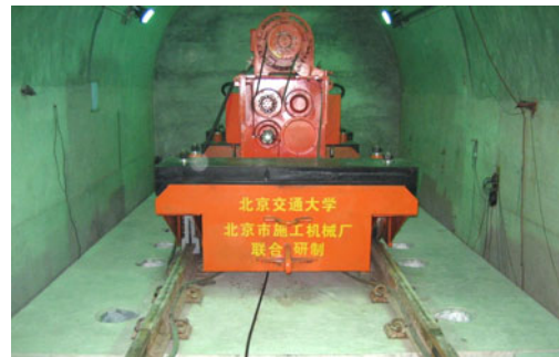
Fig. 4 Unbalanced shaker SBZ30 used for the dynamic simulation
